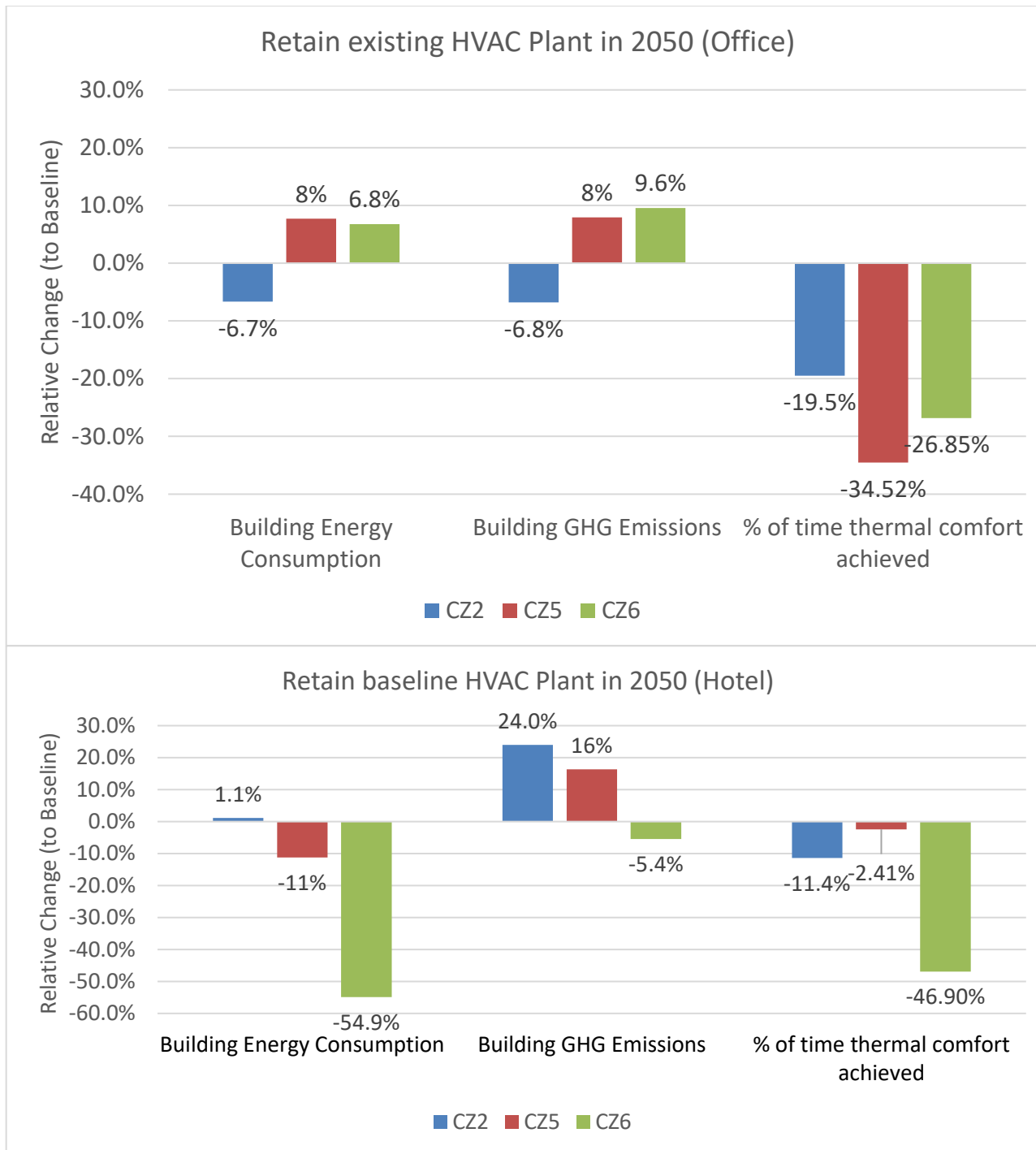
Figure 47. Impact of retaining HVAC plant sized using baseline climate files in a 2050 climate scenario. Daytime building (top) versus overnight building (bottom).
